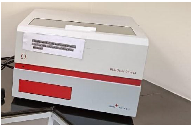
Fig. 1: Multimode microplate reader used for MTT assay
